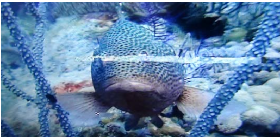
Figure 3 Picture failure caused by LTE interference
