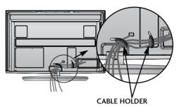
Install the CABLE MANAGEMENT CLIP as shown.
